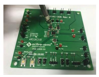
Figure 4-Measuring output voltage ripple
