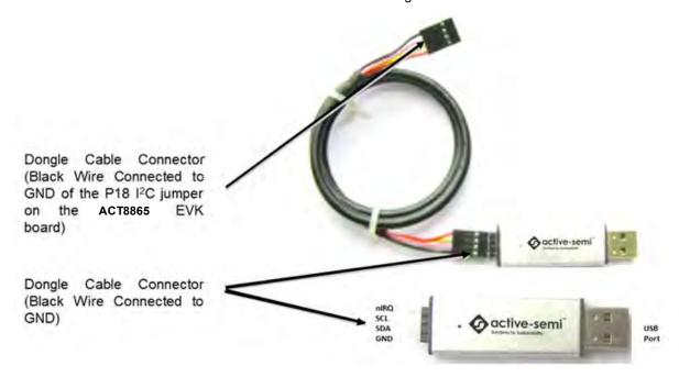
Figure 3 - USB-TO-I2C Dongle Connection
